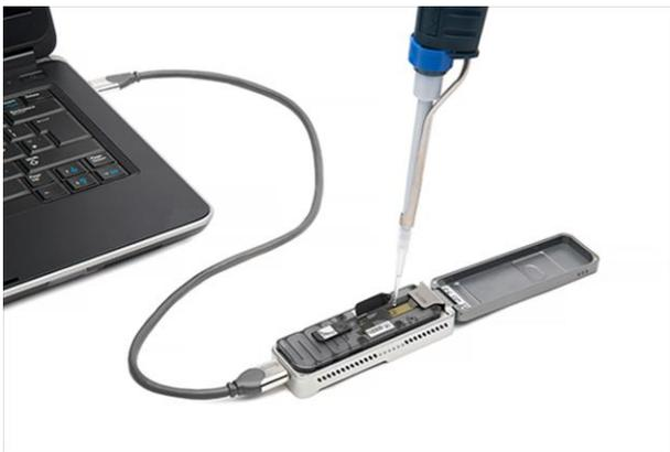
図 6. MinION (Oxford Nanopore Technologies)
