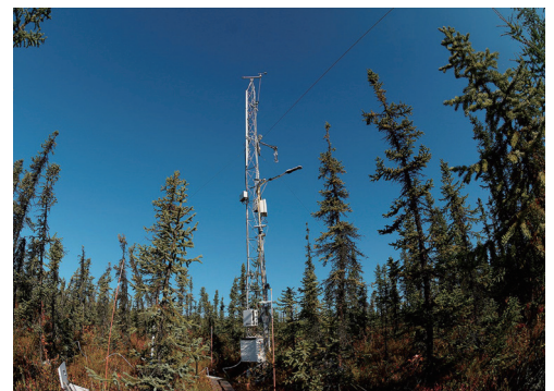
A tower installed in a black spruce forest on permafrost in Fairbanks, Alaska, monitors CO 2 exchange and environmental conditions in 30-minute intervals.
