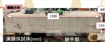
Fig.2\_Beam Specimen Used in The Test
