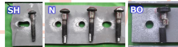
Fig. 3 Several failure modes confirmed in the test
