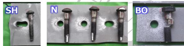
Fig. 2 Several failure modes confirmed in the test
