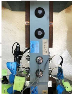
Fig. 2 Tensile test of joints made of SBHS
