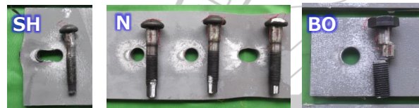
Fig. 2 Several failure modes confirmed in the test
