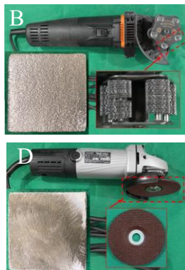
Fig. 3 Surface treatment by power tools
