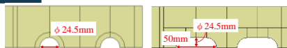
Normal hole (NH) Slotted hole (SH) Fig 3. hole shape of main plate
