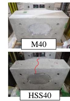
Fig.7 Cracks in mortar around the stud
