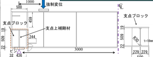
Fig. 2 Plate Girder End with Fulcrum Block
