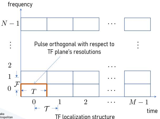
time resolution (symbol interval) (subcarrier spacing)  $g_{m,n}(t) = g(t-m\mathcal{T})e^{j2\pi n\mathcal{F}(t-m\mathcal{T})}$   $0 \leq m \leq M-1, 0 \leq n \leq N-1$
