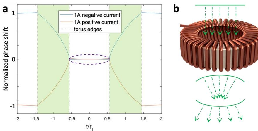
Figure 1. a) Calculated phase profiles for an electron plane wave passing an ideal toroidal solenoid. The light green areas within the dotted vertical lines represent regions inside the torus volume where magnetic field is present. The dotted ellipse highlights the central hole of the torus which is field-free yet exhibits lensing curvature. b) Schematic of how a toroidal solenoid coil can behave as a concave or convex lens for particles with negative or positive charge.
