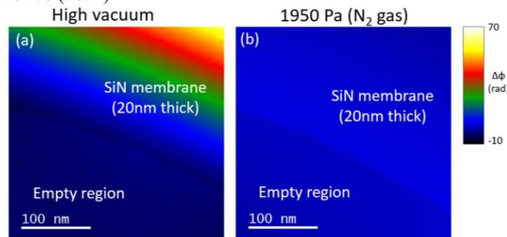
Fig. 1. Phase maps, reconstructed from 300kV off-axis holograms, from a 20nm SiN membrane. (a) Standard high vacuum case. (b) Same film region as (a) but with 1950 Pa N<sub>2</sub> gas in the specimen area. There is a clear, charging-induced phase ramp in (a), which has been substantially reduced by the introduction of N<sub>2</sub> gas in (b).
