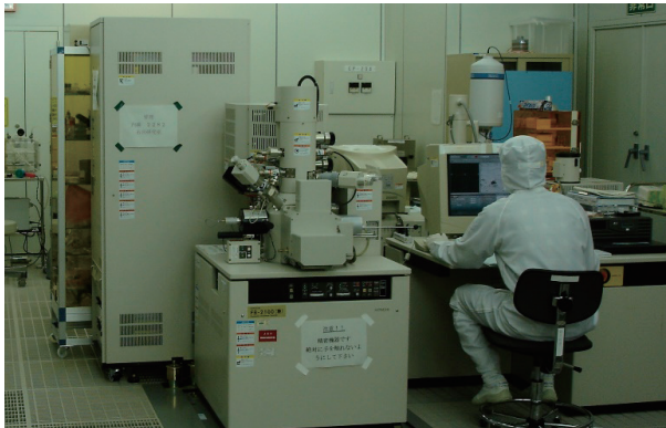
Focused ion beam apparatus installed in the clean room
