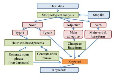
Figure 2. Generating keyword algorithm
