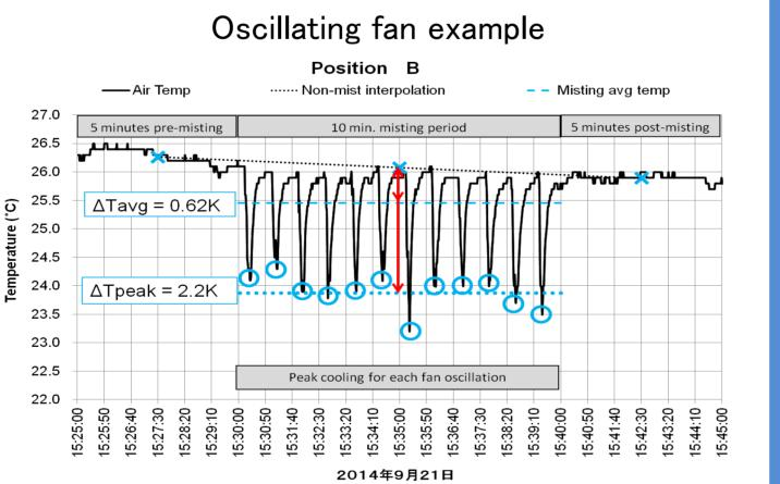
Fast response sensor temperature measurements example data • Time-averaged temperature drops are small due to
