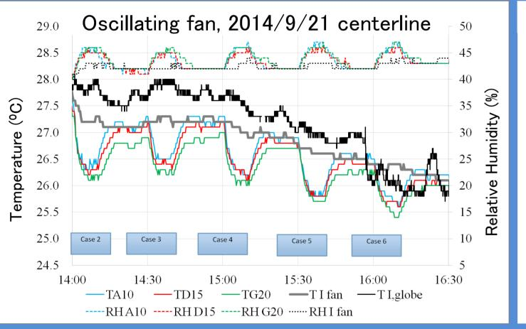
Slow response sensor temperature and humidity measurements
