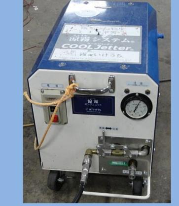
1 pump supplies 6 mist fans Pressure = 6MPaSpray volume = 510l/h Electric power = 750W
