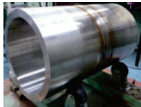
Ring specimen for welding
